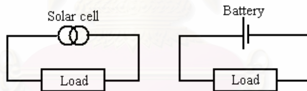
Figure 3.3 The solar cell may replace a battery in a simple circuit.
