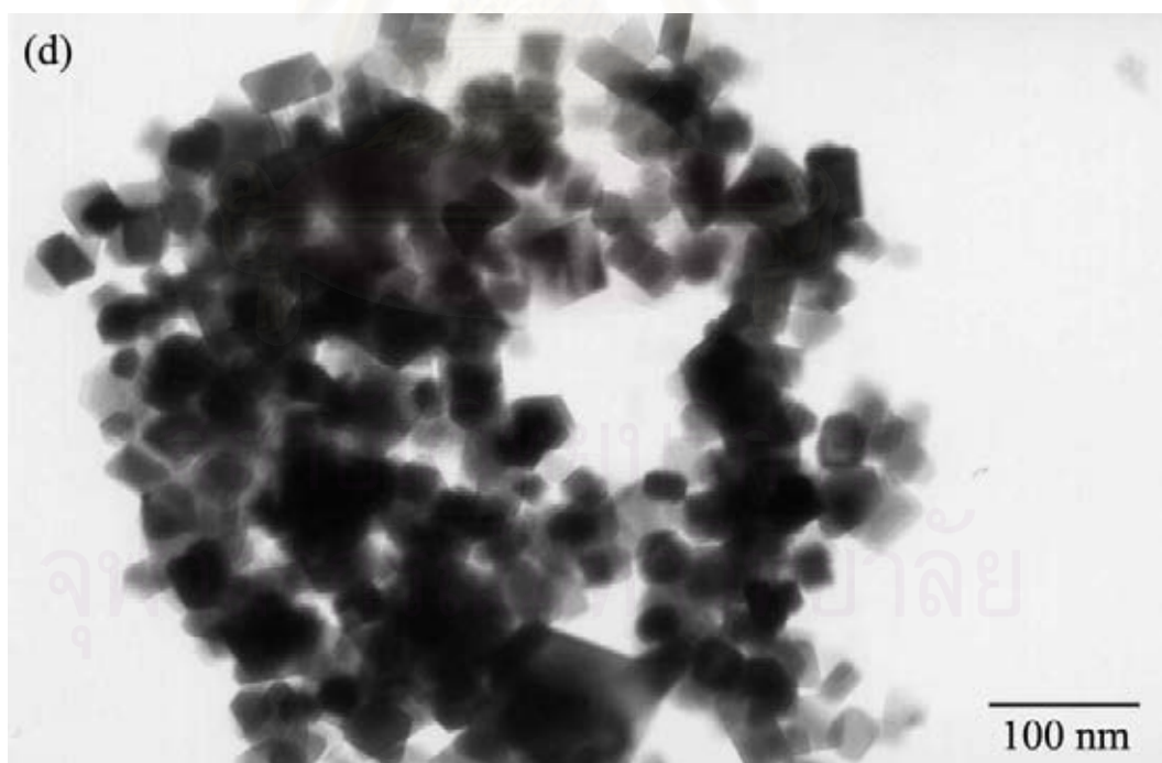
Figure 5.5(d) TEM photograph of the zinc chromite product prepared at reaction heating rate of 1.0°C/min after calcined at 1000°C (x150000)
