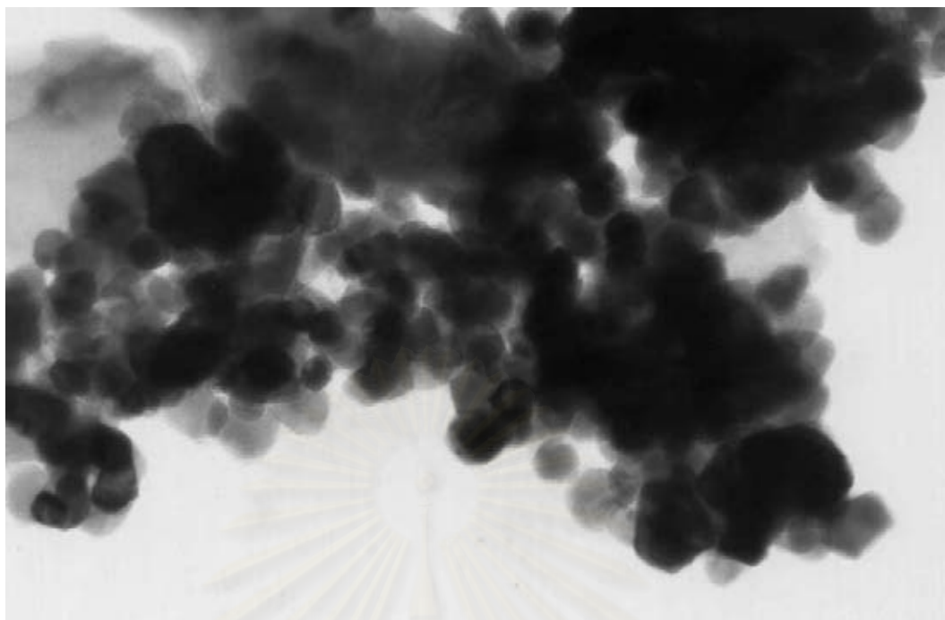
Figure 5.7 TEM photograph of the undetermined intermediate product prepared at reaction heating rate of 2.5°C/min (x150000)
