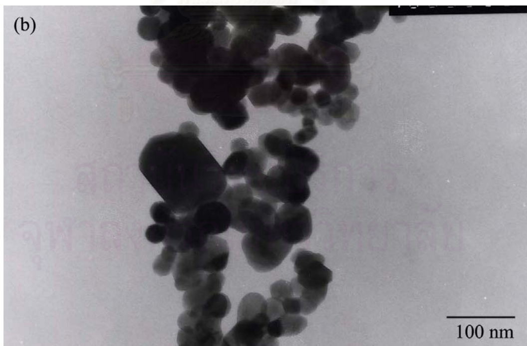
Figure 5.17(b) TEM photograph of the zinc ferrite product prepared at reaction heating rate of 2.5°C/min after calcined at 600°C (x150000)
