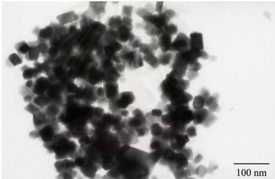
Figure D.2 TEM photograph of calcined zinc chromite at calcination temperature 1000^\circ\text{C} (x150000)
