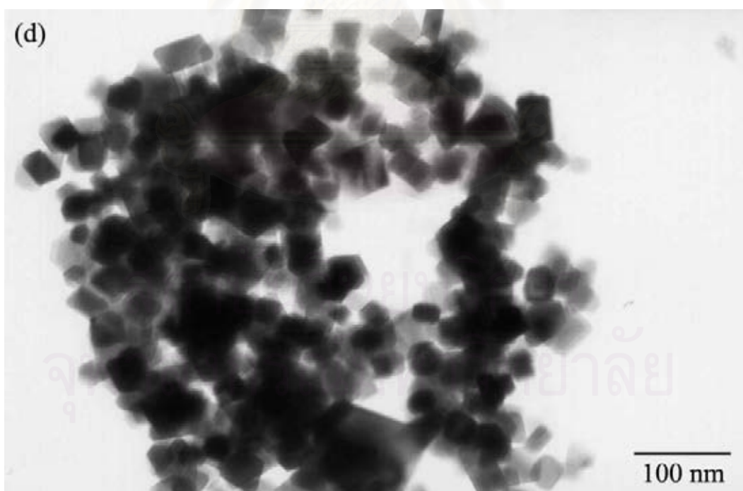
Figure 5.4(d) TEM photograph of the zinc chromite product prepared at reaction heating rate of 2.5°C/min after calcined at 1000°C (x150000)
