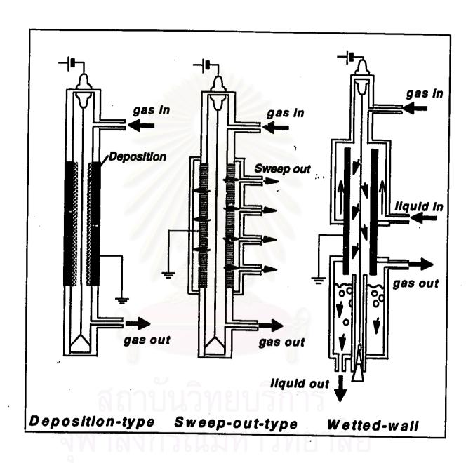
Figure 3.2 Concepts of corona-discharge reactor
