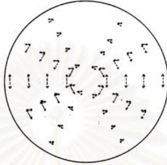
Figure 2-14 : The arrangement of induced dipoles in a tangentially polarizable spherulite which will contribute to Hv scattering. [Stein, R.S. 1960]
