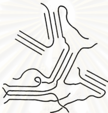
Figure 2-2: The fringed micelle model. Each chain meanders from crystallite to crystallite, binding the whole mass together. [Sperling, L.H. 2001]
