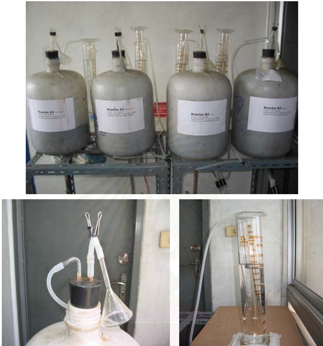
Figure 3.1 Configuration of the simulated landfill fermentation of organic waste reactors
