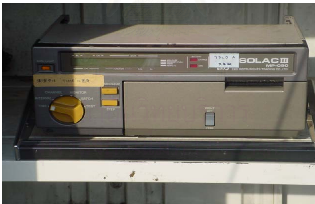
Figure 3.7 Data collector (SOLAC III)
