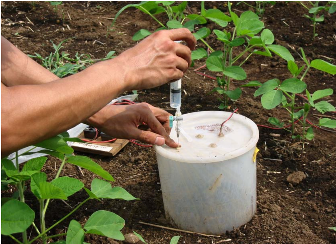
Figure 3.8 Demonstration of sampling technique from closed chamber.
