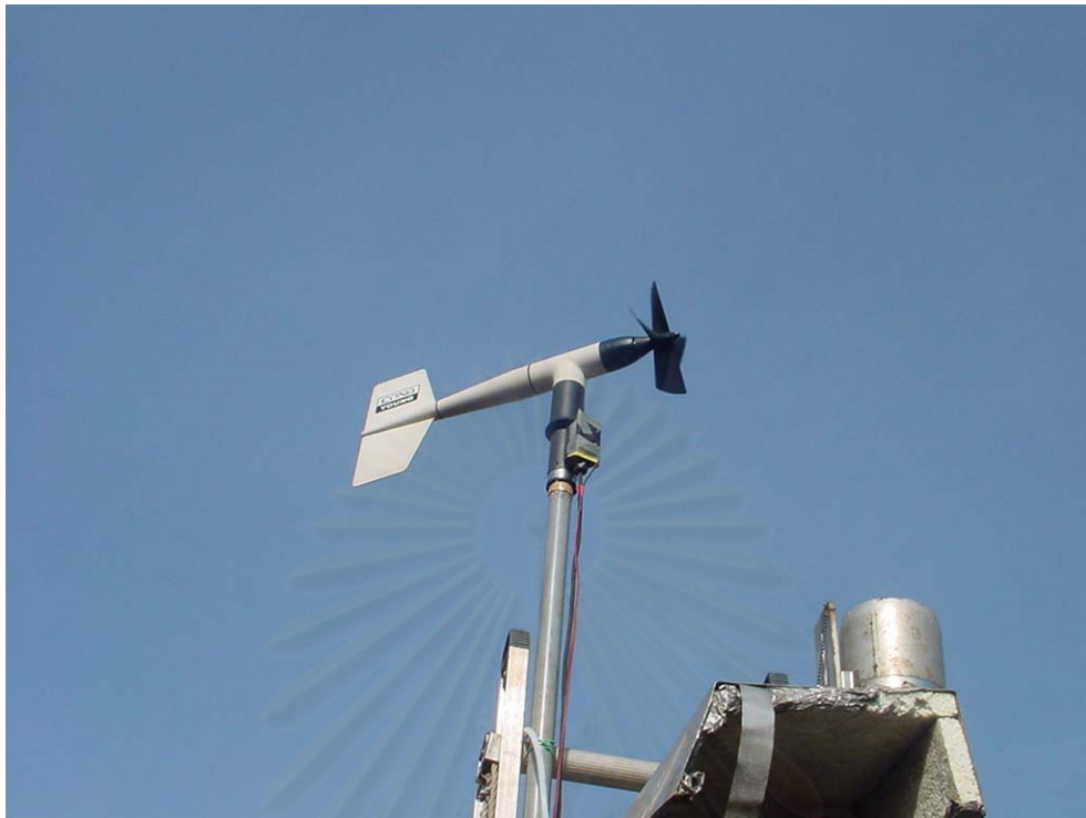
Figure 3.20 Anemometer at the top of tower.
