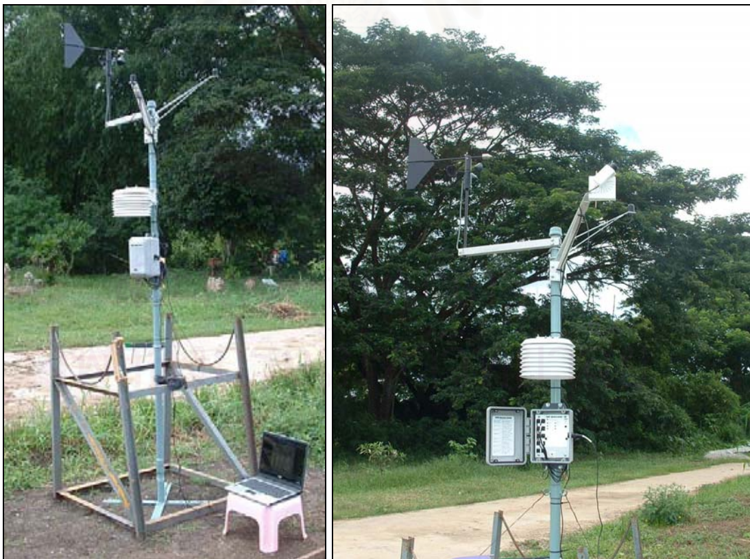
Figure 3.5: The HOBO weather station with smart sensors.
