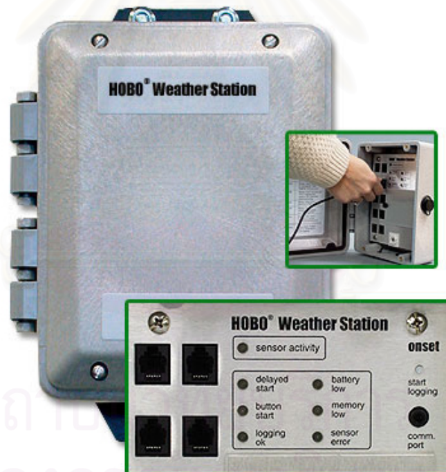
Figure A1: HOBO Weather station (Data Logger).
