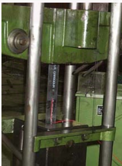
Figure A.1 Static test on CFRP laminates
