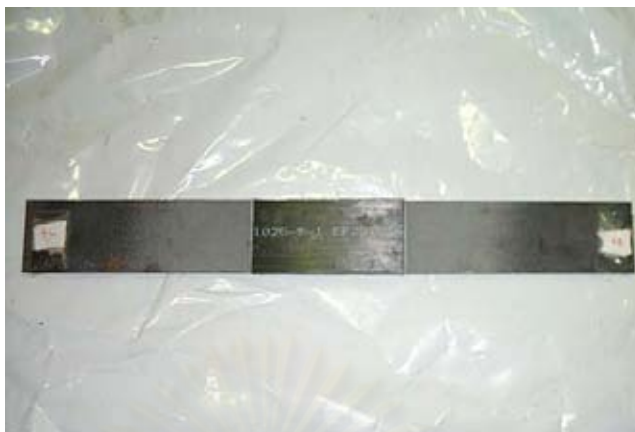
Figure 4.8 CFRP-steel double strap joint specimen (Preliminary test)
