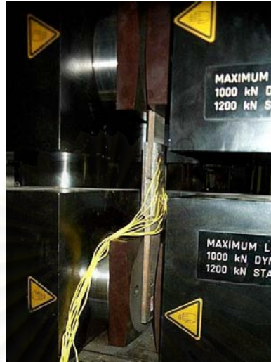
Figure 4.11 Test setup for double-strap joint specimens
