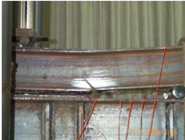
Figure 2.1 Typical fatigue failure from welded cover plate details
