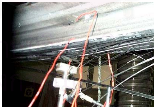
Figure 7.2 FRP plate rupture failure mode at midspan
