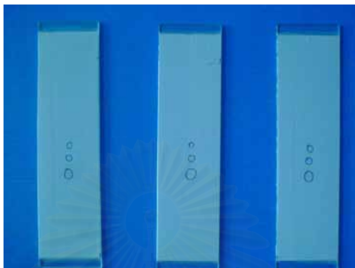
Figure F18 TLC testing of synthesized silica gel at aging pH 3 mixed with 10% \text{Na}_2\text{SO}_4 .
