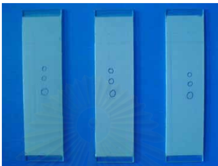
Figure F16 TLC testing of synthesized silica gel at aging pH 3 mixed with 10% BaSO 4 .
