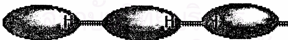
Figure 3.19 The random orientation of monomers in the polymer chain [157]
