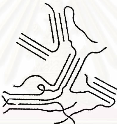
Figure 3.8 The fringed micelle model [163]
