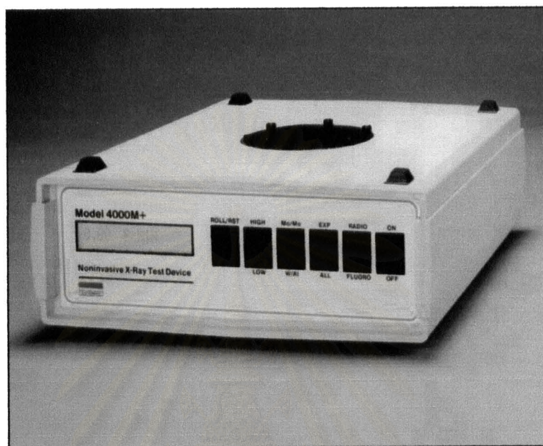
Figure 3.4 Ionization chamber (Victoreen 4000 M + )
