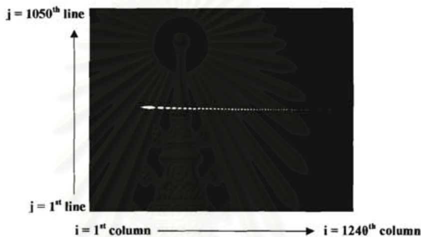
Figure 6.11: Image of the scattered light by liquid jet used for calibration.
