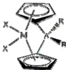
Figure 2.1 Typical chemical structure of a metallocene catalyst
