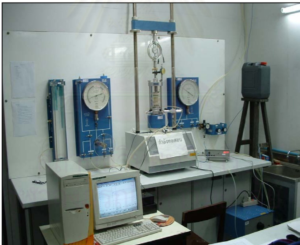
Figure 3.5: Setting of triaxial apparatus and bender elements
