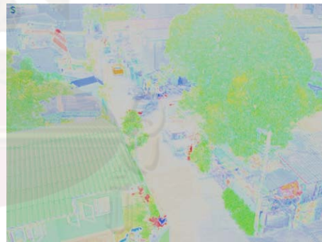
Figure 1 HSV color space image with fixed V value
