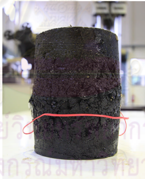
Figure 3.17 Typical failure mechanism of asphaltic concrete under S-UC test
