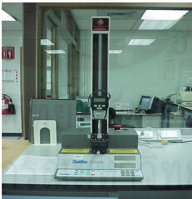
Figure 3.3 The shear strength test instrument
