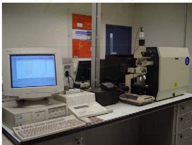
Figure 4.11 Raman Microscope (Renishaw Ramascope System 2000)
