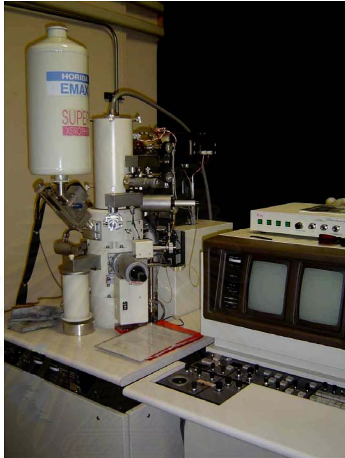
Figure 4.7 Field Emission Scanning Electron Microscope (FESEM)
