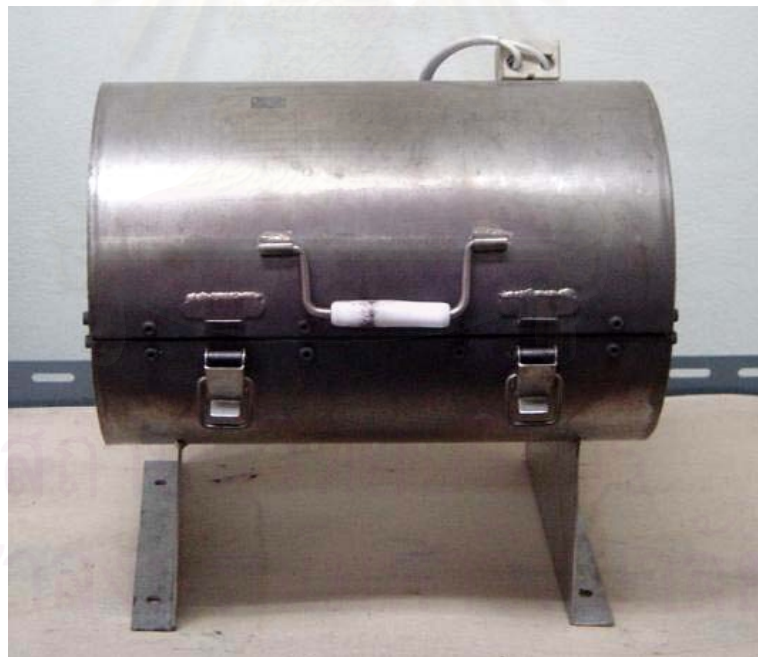
Figure 4.2 Tube furnace reactor
