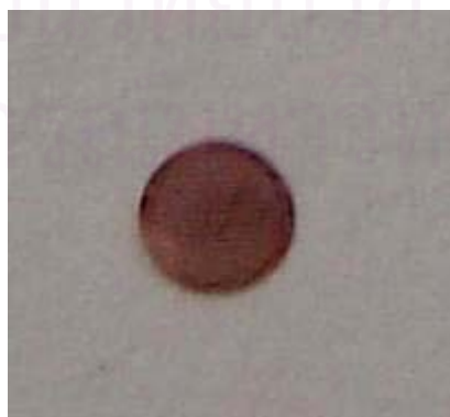
Figure 4.9 Copper grid coated with carbon films for Transmission Electron Microscopy
