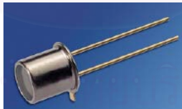
Figure 3.20: Picture showing the BPX-65 PIN diode[48].
