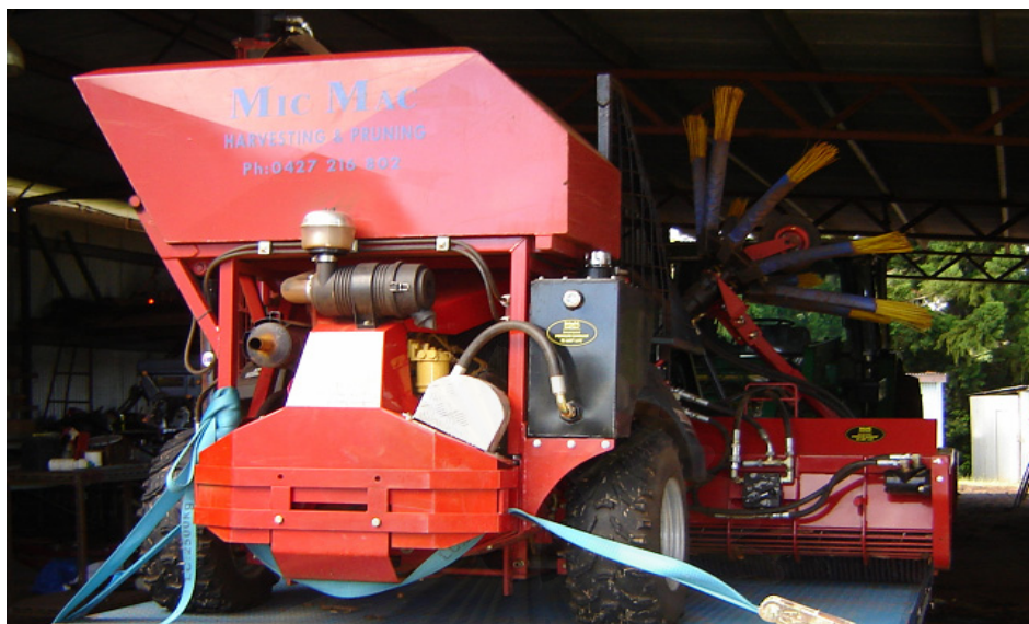
Figure 2.7 Macadamia nut sweeper and blower machine
