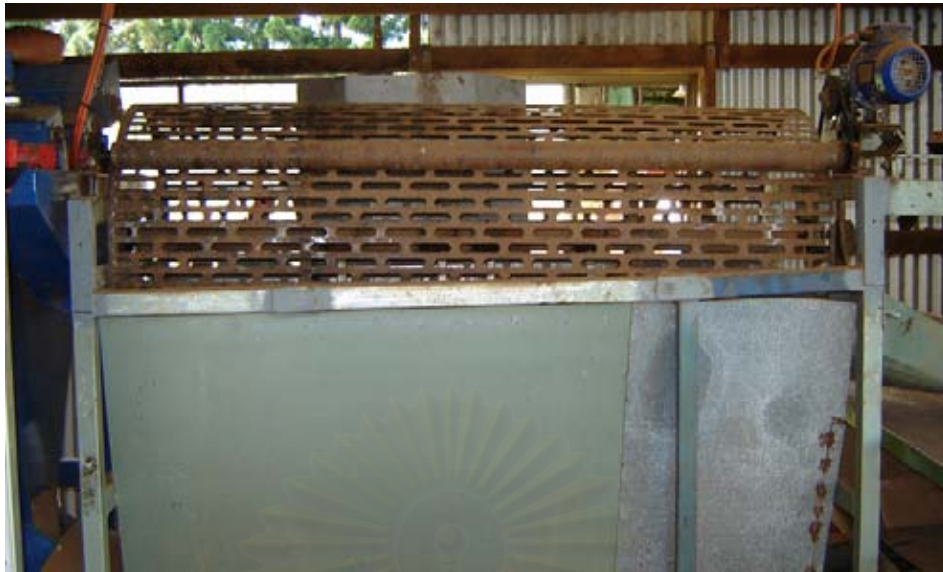
Figure 2.10 The size grading of macadamia nuts in shell
