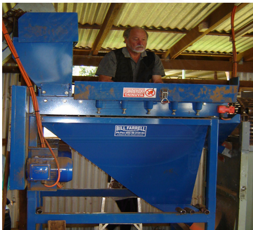
Figure 2.9 Dehusking machine of macadamia nuts
