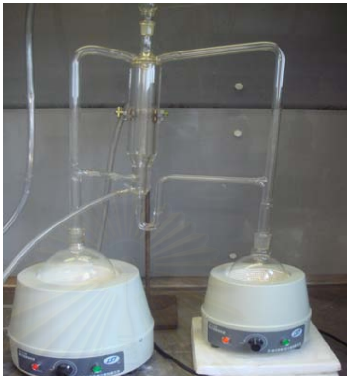
Figure 3.5 Modified Likens-Nickerson simultaneous distillation and extraction apparatus
