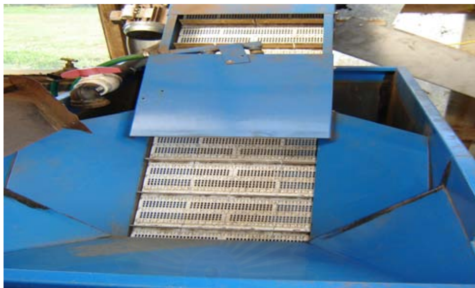
Figure 2.11 The nut in shell grading by floating
