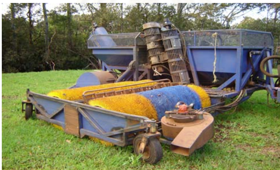
Figure 2.8 Macadamia nuts harvesting machine
