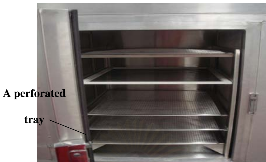
Figure 3.2 Heat pump dryer (UNSW, Australia)
