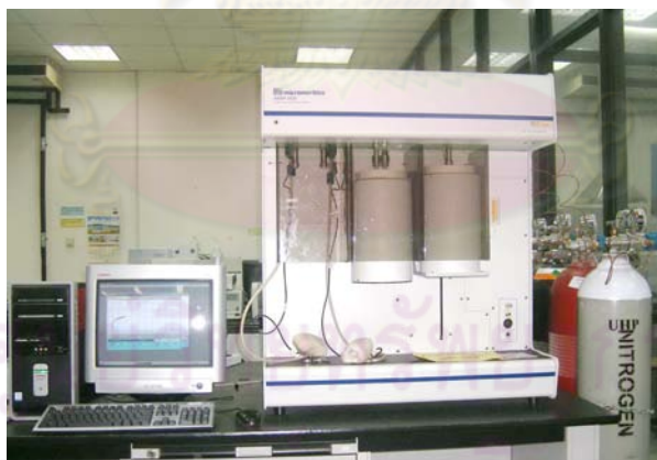
Figure 3.3 Surface area and porosity analyzer
