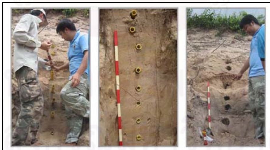
Figure 3.7. Methodology used to collect sample for define absolute age by optically stimulated luminescence (OSL) dating. Collecting the samples from the top of profile dune is every 0.15 m.
