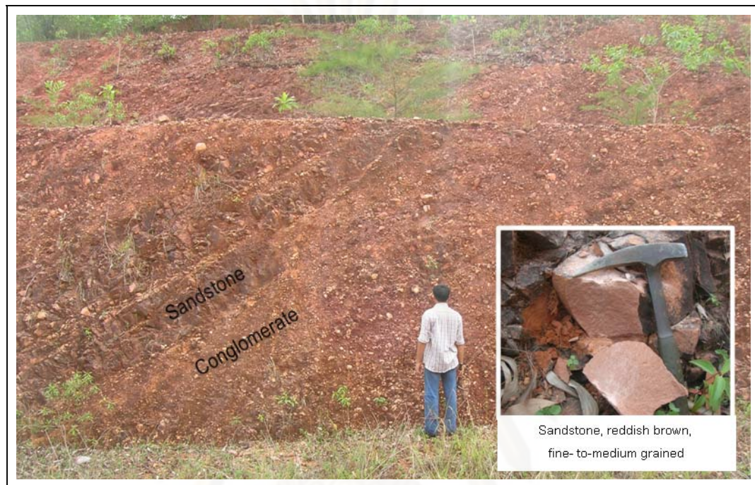
Figure 2.5. Reddish brown sandstone interbedded with conglomerate at highway no.3114, northern part of the study area.
