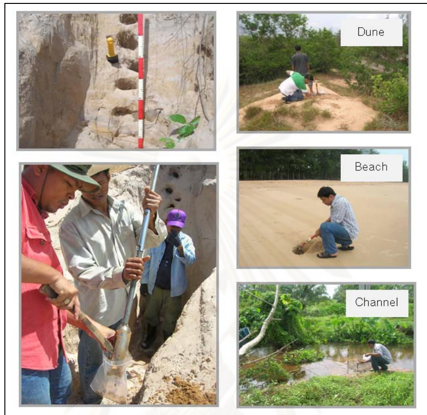
Figure 3.6. Methodology used to collect sample for analysis grain size to define environment deposits, by pitting and auguring.
