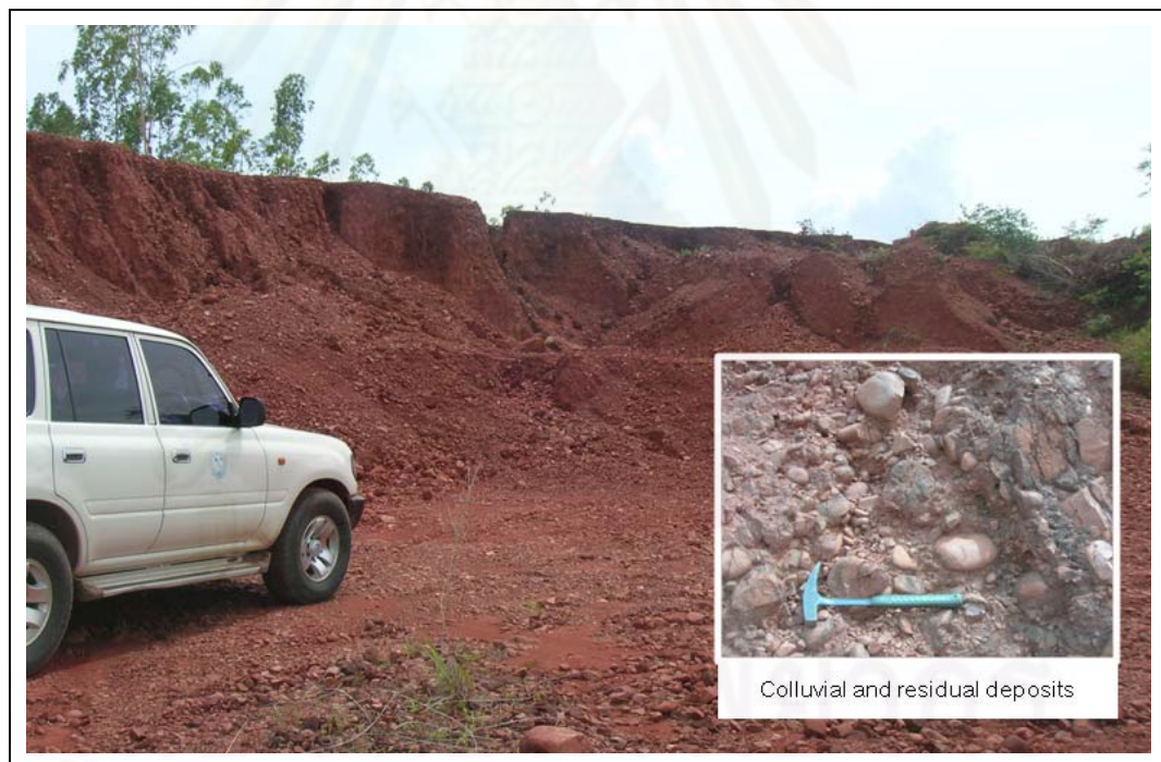
Figure 2.6. Rock fragments of quartzite, sandstone, siltstone, granite, sand and silt matrixes of colluvial and residual deposits in the northern part of the study area.
