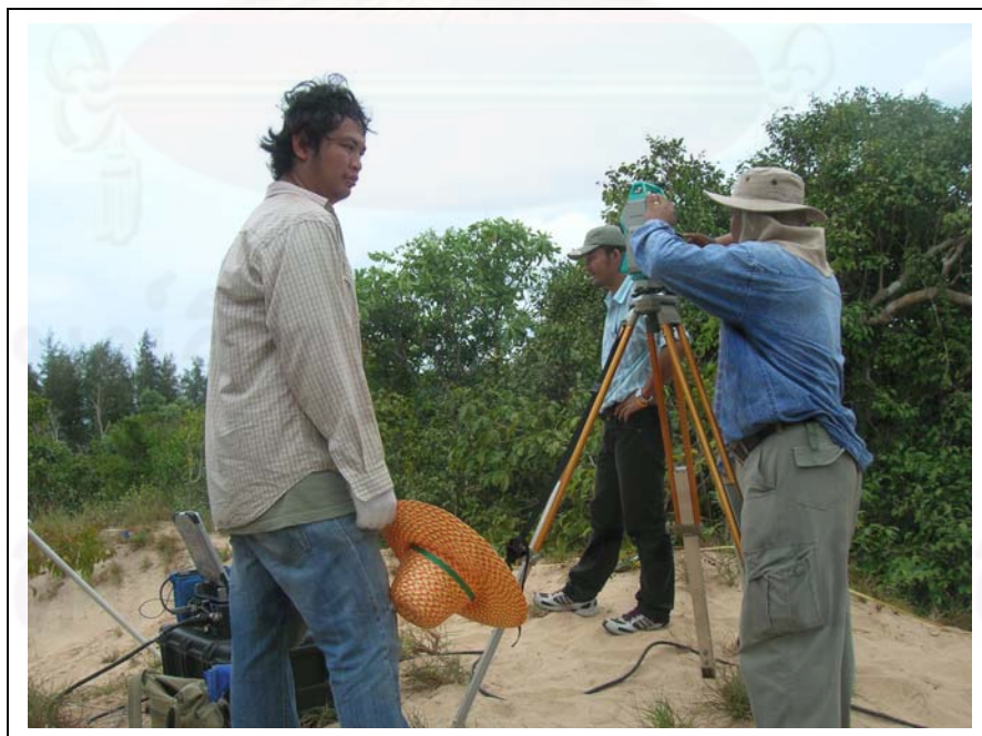
Figure 3.3. Topographic survey for profiling dune morphology along GPR lines.
