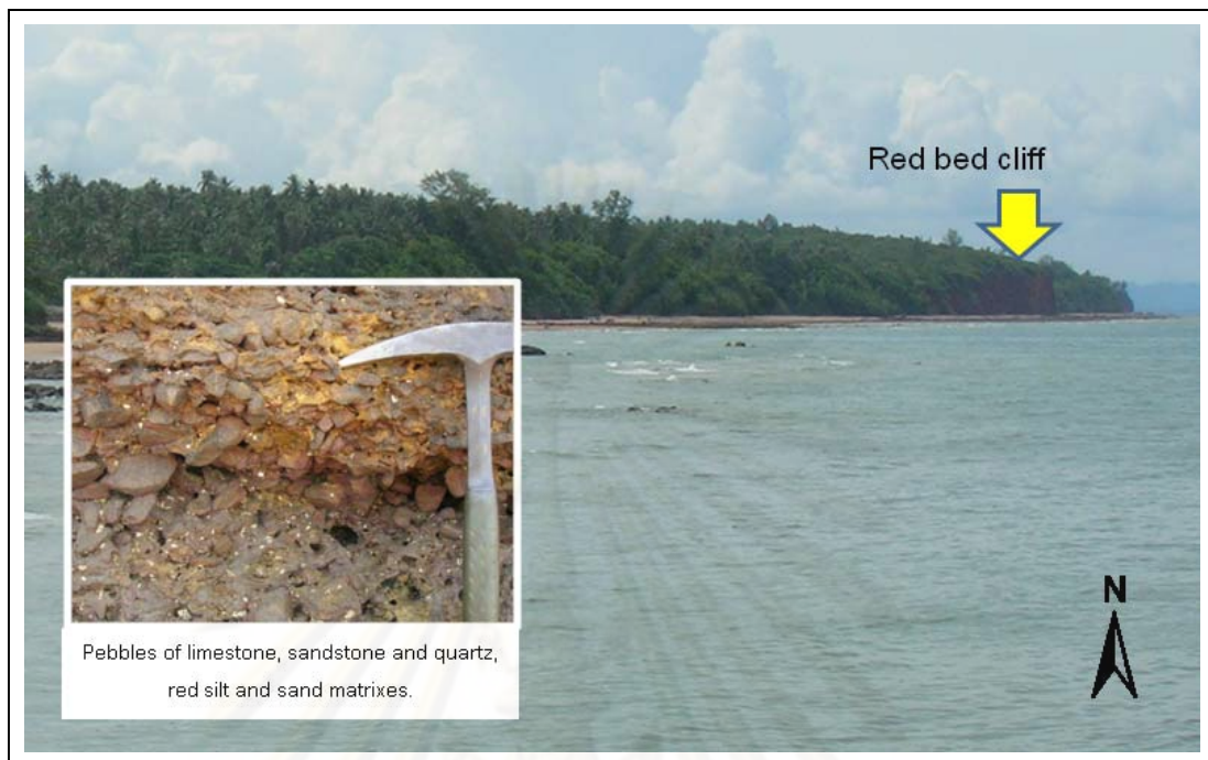
Figure 2.4. The red bed cliff near the coast in the northern part of the study area. Rocks are composed of basal conglomerate, pebbles of limestone, subangular to angular, sandstone and quartz, sub-rounded to rounded with calcareous matrix and cement.
