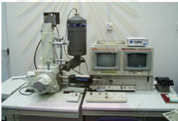
**Figure 4.6:** Scanning electron microscope (SEM)
