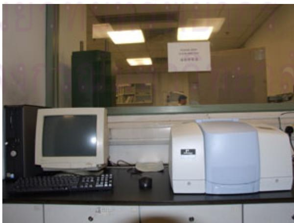
**Figure 4.7:** Fourier transform infrared spectrometer
