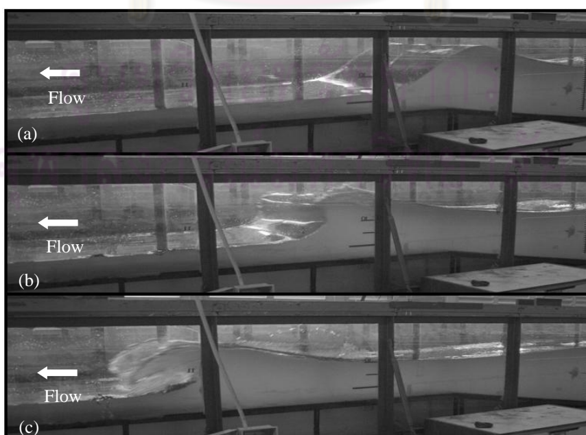
Figure 3.3 Simulated tsunami waves and wave breaking
