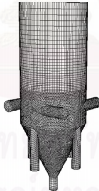
Figure IV-5 Grid system of Hydrocyclone II
