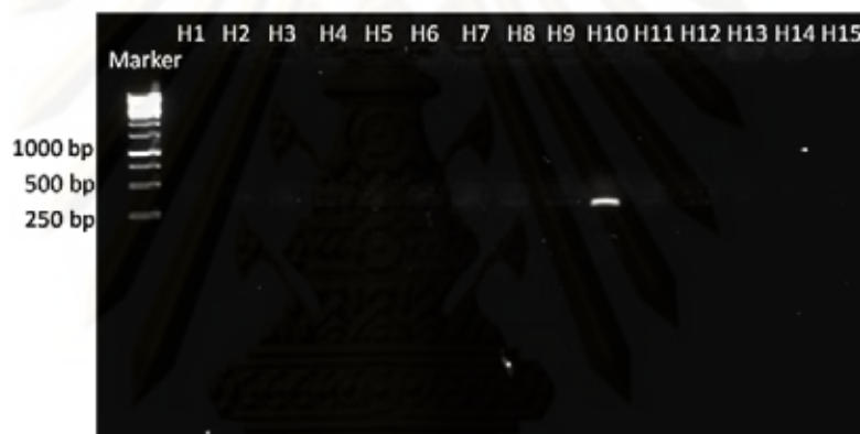
Figure 11 : Subtype identification by PCR with H1-15 subtyping primers of sample No. LM 4754. The sample was positive as H10 subtype (311 bp).
