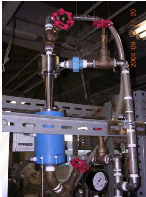
Figure 4.2 (a) Hydrocyclone and the dust box
