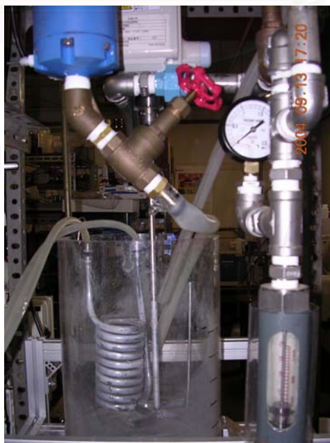
Figure 4.2 (b) Tank, control valve, impeller, flow meter and pressure gauge
