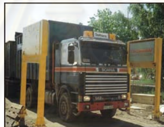
AT-900 Truck Monitoring Systems as Normally used for Scrap Monitoring.
