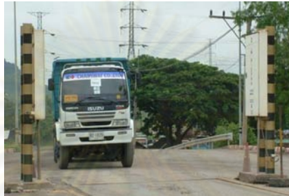
BICRON ASM -6000E Truck Monitoring Systems as Normally used for Scrap Monitoring
