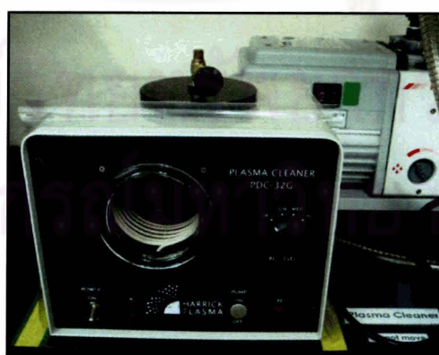
Figure 3.6 The air plasma cleaner.
