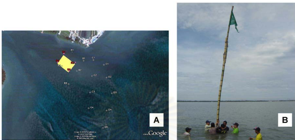
Figure 5.16 (A) Reserve area (yellow) and stations used during field data collection, (B) Installing of reserved area by using bamboo poles and flags on the sandbar
