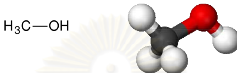
Fig 4-11 Molecular structure of methanol; 2-dimension (left), 3-dimension (right)
