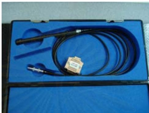
**Figure 3.5** The pencil ionization chamber
