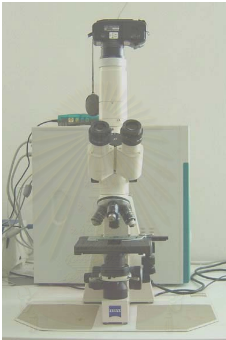
Figure 1 Compound microscope Zeiss model Axiostar attached with digital camera Sony Cyber-shot DSC-S85
