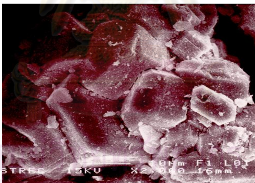
Figure 5.11 (a) The SEM images showed fresh Ni/γ-Al 2 O 3 commercial catalyst.
