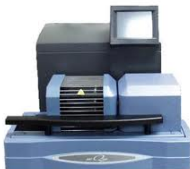
Figure 3.7 Instrument of thermogravimetric analyzer-differential scanning calorimeter.
