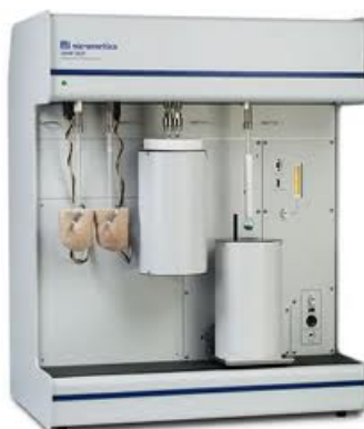
Figure 3.6 Instrument of nitrogen physisorption measurement.
