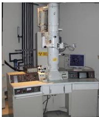
Figure 3.5 Instrument of transmission electron microscopy.
