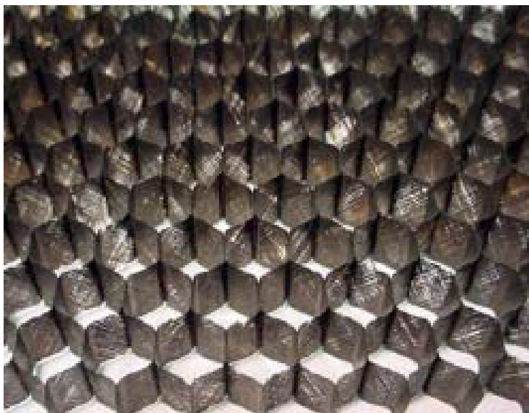
Figure 2.9: Carbon fiber honeycomb core
