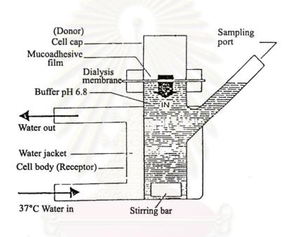
Figure 25 Schematic diagram of the apparatus for the in vitro release and penetration studies
