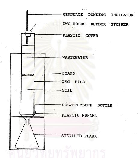
Figure 1 Typical soil column used in the experiment.
