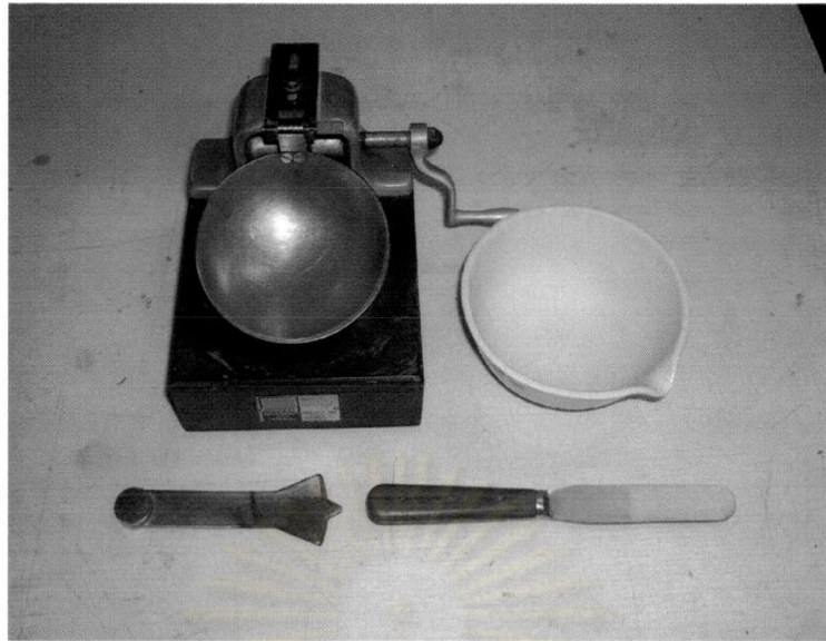
Fig. 3.4 Atterberg's limit test equipment
