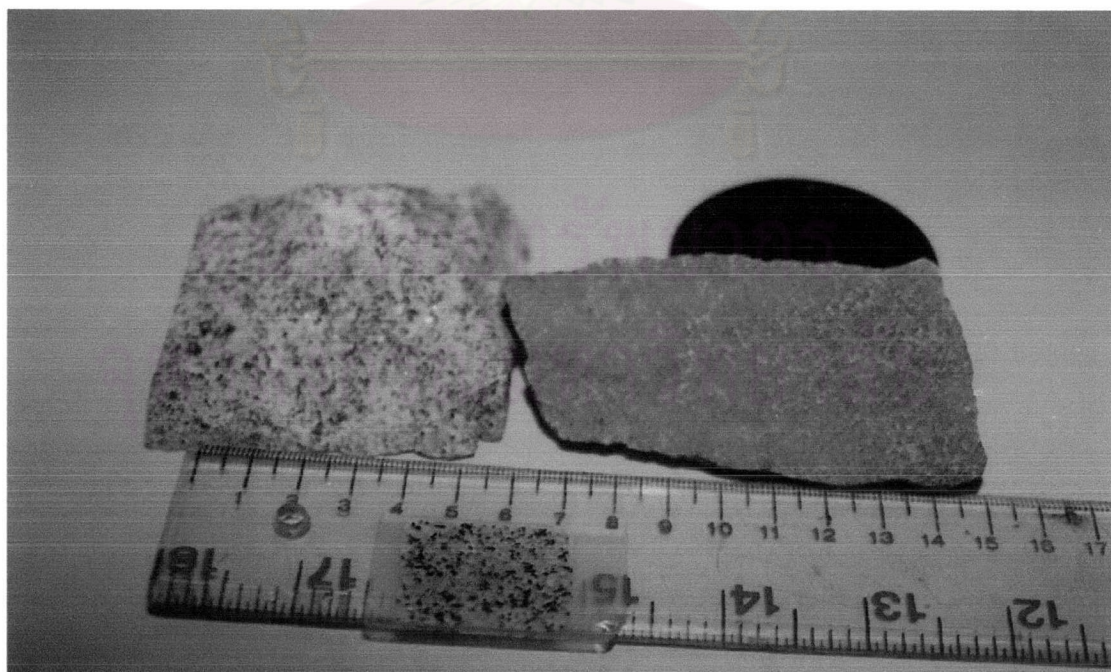
Figure 3.27 Specimen and staining slab of hornblende-biotite granodiorite.
