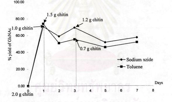
Conditions: chitinolytic enzymes (8 U) in McIlvaine buffer pH 3 (0.1 M, 20 mL). The mixture was incubated at 45 °C and chitin was added after 1 and 3 days of incubation. Dashed lines indicate the addition of chitin in fed batch technique.
