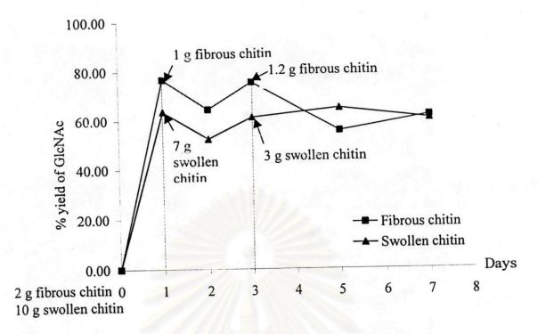
Conditions: chitinolytic enzymes (8 U for hydrolysis fibrous chitin and 40 U for hydrolysis swollen chitin) in McIlvaine buffer pH 3. The mixture was incubated at 45 °C and chitin was added after the 1 and 3 days of incubation.
