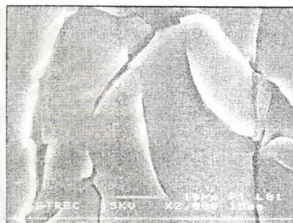
Unvulcanized natural rubber sheet after UV exposure for 8 h.
