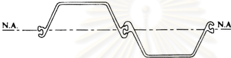
(b) Actual neutral axis location along line of interlocks and as commonly used in European practice.
