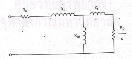
Fig. 3.1 Induction Motor Equivalent Circuit
