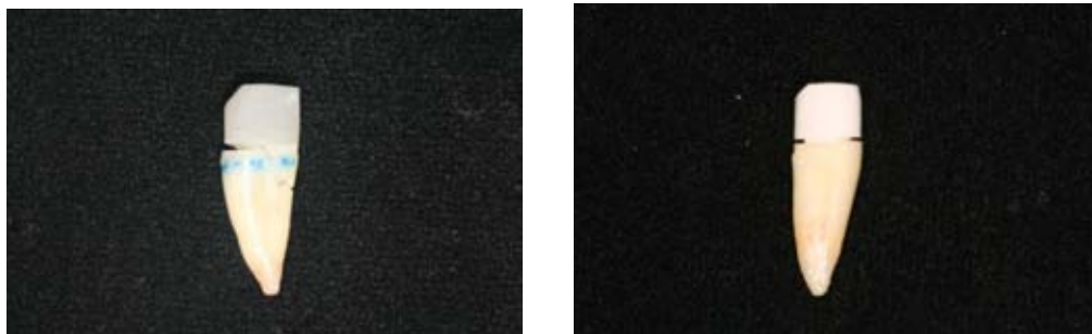
Fig. 9 Fracture mode of specimen which was non-repairable and repairable
