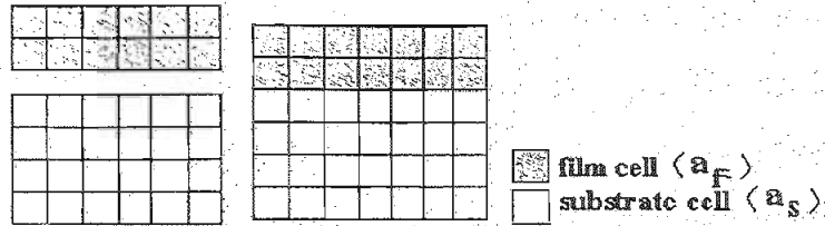
Fig 2.18 Growth of an epilayer on a perfectly lattice-matched substrate.
