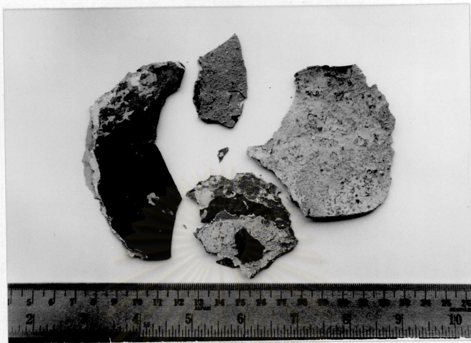
Figure 2-1 Scrap-paints which came off the steel plate of a vessel.
