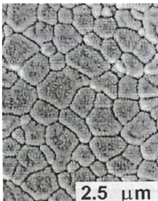
Fig.2.7 SEM microstructure of a 2.5 mol% Y-TZP material sintered 1 h at 1500°C
