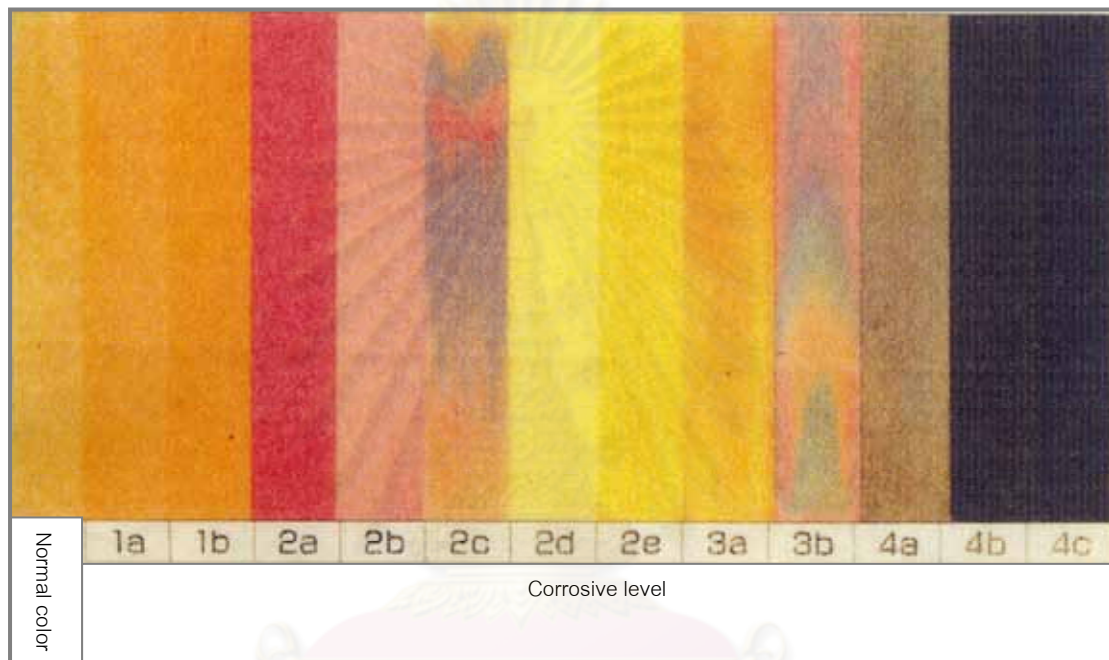
Figure B9 ASTM corrosion standards.
