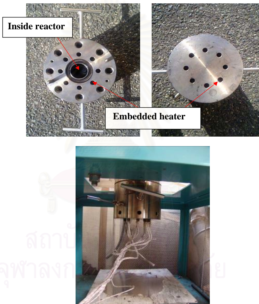
Figure 4.2 Autoclave reactor and 8 embedded heaters
