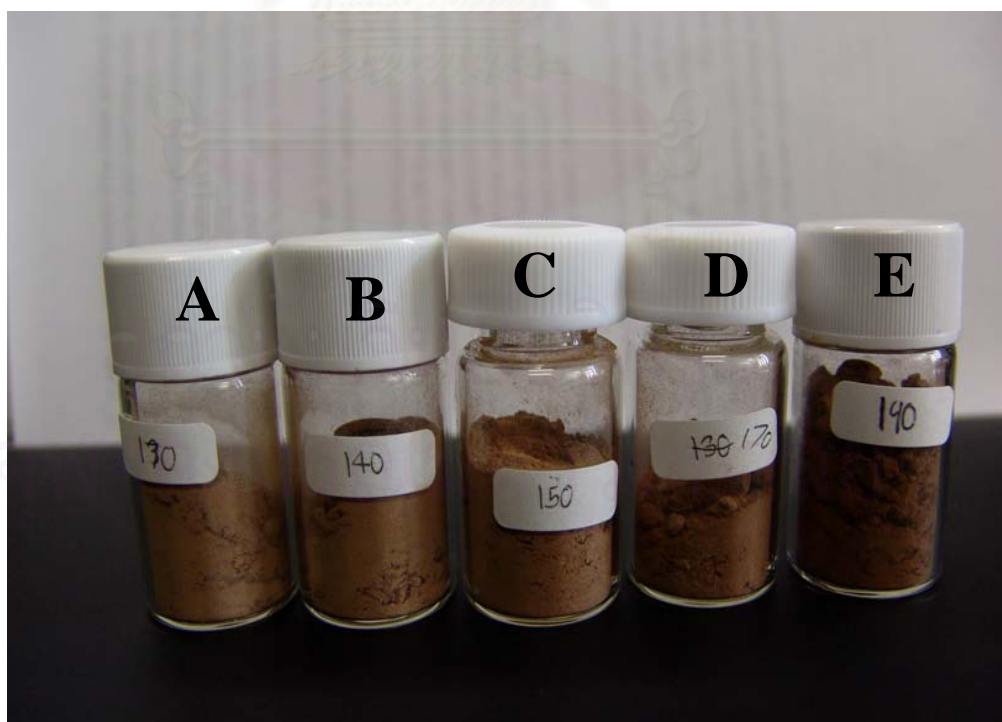
Figure 5.6 The solid samples after hydrothermal pretreatment at temperature on (A) 130, (B) 140, (C) 150, (D) 170, and (E) 190 °C
